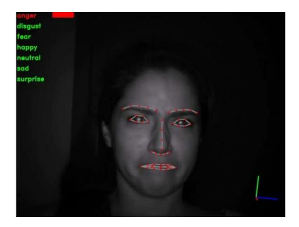
The device detects anger on the driver's face. Credit: EPFL-LTS5 & PSA
