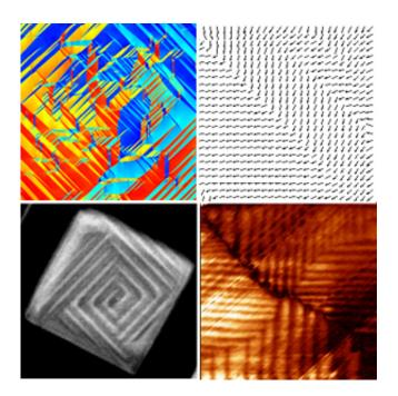
A simulated polarization pattern (top left), polarization vectors within the simulation (top right), and polarization patterns visualized using transmission electron microscopy (bottom left) and piezoresponse force microscopy (bottom right) in the ferroelectric material barium titanate. Credit: American Physical Society
