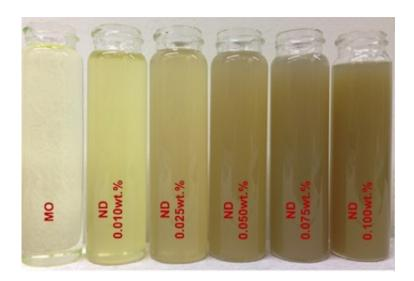
Mineral oil combined with nanodiamonds is more effective than other nanofluids for heat-transfer applications, according to researchers at Rice University. The researchers tested nanodiamonds in mineral oil at concentrations up to 0.1 percent weight to see how well it would transfer heat while remaining at a usable viscosity. Credit: Ajayan Group
