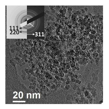
An electron microscope image shows diamond nanoparticles suspended in oil. The inset shows the diffraction planes of the particles. Credit: Ajayan Group
