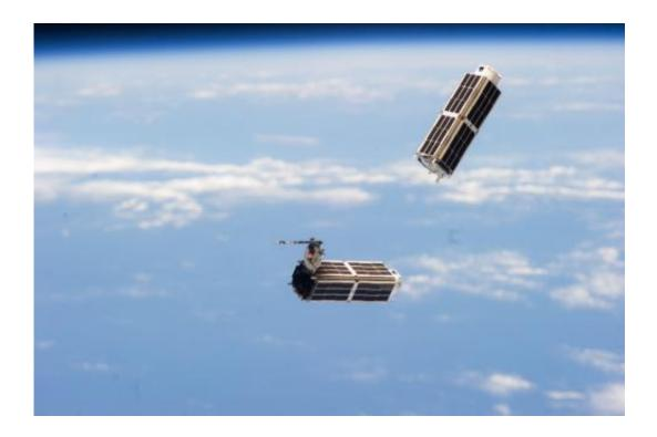
Two of the 28 Planet Labs Dove satellites that make up the Flock 1 constellation are seen launching into orbit from the International Space Station on Feb. 11. Credit: Image Credit: NASA
