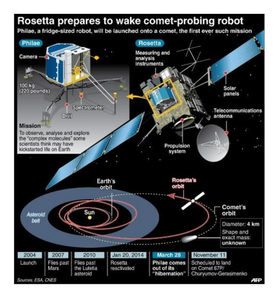
Fact files on the Rosetta probe and the Philae robot it will send down to land on and analyse a comet. (130 x 140mm)
