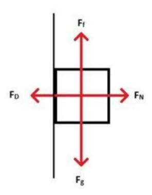
A free-body diagram showing forces acting on the centre-of-mass of a vehicle travelling on a vertically banked track. Credit: University of Leicester
