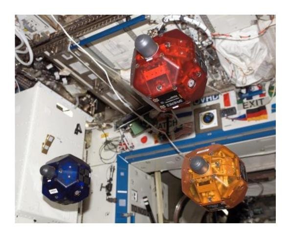
Three satellites fly in formation as part of the Synchronized Position Hold, Engage, Reorient, Experimental Satellites (SPHERES) investigation. This image was taken aboard the International Space Station during Expedition 16 in the U.S. Destiny laboratory module. Credit: NASA
