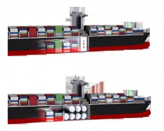
Above is a container ship having a box-shaped pressure vessel as a fuel tank, and below are traditional cylindrical fuel tanks. Credit: KAIST
