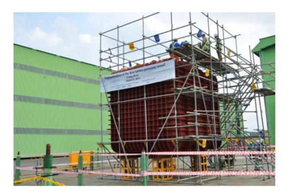
This is a photo of the prototype of a box-shaped pressure tank. Credit: KAIST
