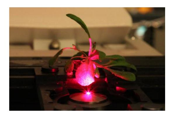
Nanomaterials can enable plants with novel and augmented functions. This Arabidopsis plant with carbon nanotubes inside its leaves has augmented light energy capture and could act as a photonic biochemical detector. Credit: Juan Pablo Giraldo
