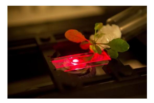
Imaging the fluorescence of carbon nanotubes inside leaves of an Arabidopsis plant using a single particle near infrared microscope. Credit: Bryce Vickmark
