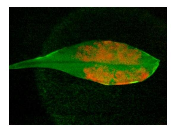
Near infrared fluorescence of carbon nanotubes (orange) infiltrated inside leaves (green) could boost photosynthesis and enable the detection of biochemicals and pollutants. Credit: Juan Pablo Giraldo and Nicole M. Iverson
