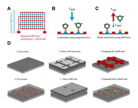
Schematic A shows the chip layout, with circular nickel pads (blue), which can be magnetized by an external magnet flanked by interdigitated gold electrodes (red). Schematic B shows paramagnetic beads introduced to the chip surface by microfluidics and loaded onto the magnetic pads by magnetic manipulation, facilitating the formation of bead surface tethers via antibody-antigen
