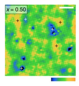
Images obtained through scanning tunneling spectroscopy show the transformation of a compound of strontium, iridium and oxygen—part of a mysterious class of materials known as spin-orbit Mott insulators. By introducing
