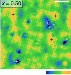
Images obtained through scanning tunneling spectroscopy show the transformation of a compound of strontium, iridium and oxygen—part of a mysterious class of materials known as spin-orbit Mott insulators. By introducing
