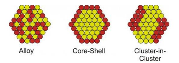
A schematic shows different nanoparticle configurations possible with a new technique to create custom bimetallic nanoparticles.
