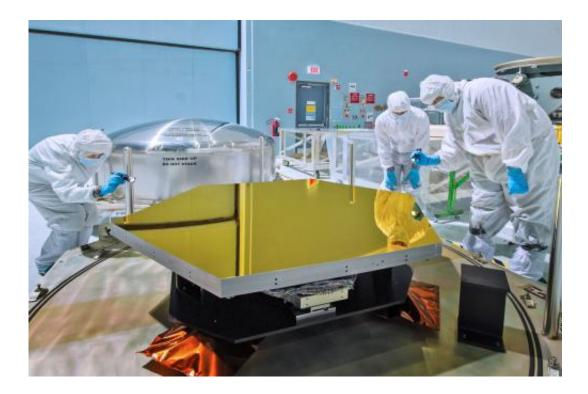
Technicians and scientists check out one of the Webb telescope's first two flight mirrors in the clean room at NASA's Goddard Space Flight Center in Greenbelt, Md. Credit: NASA/Chris Gunn
