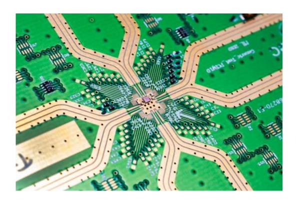
Imec, in collaboration with Vrije Universiteit Brussel, Brussels, Belgium, presents the world's first 79 GHz radar transmitter implemented in plain digital 28nm CMOS. With an output power above 10dBm, the transmitter front-end paves the way towards full radar-on-chip solutions for automotive and smart environment applications.
