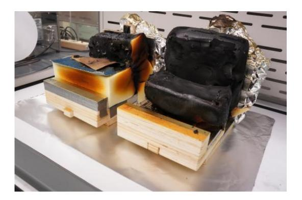
Residues of an identical foam-fabric assembly in the current (left) and in the modified (right) smoldering ignition setup (45 min test duration). The new setup promoted an increase in smoldering rate as compared to the current setup and induced transition to flaming. Credit: Zammarano/NIST
