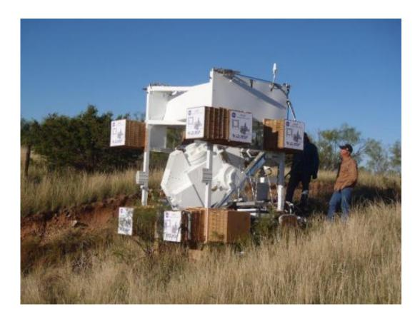
Scientists used the Wallops Arc Second Pointer to precisely point the HyperSpectral Imager for Climate Science during a balloon mission in September. Shown here after it landed, the imager collected radiance data for nearly half of its eight-and-a-half hour flight. Credit: NASA
