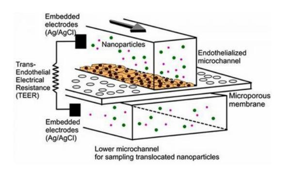
This is a schematic of an endothelialized microfluidic device that consists of twolayer microfluidic channels that are separated by a porous membrane (3  $\mu$ m pore) on which endothelial cells are grown. Credit: Credit: Kim/*PNAS*.
