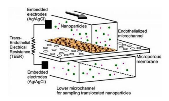
This is a schematic of an endothelialized microfluidic device that consists of two-layer microfluidic channels that are separated by a porous membrane (3 µm pore) on which endothelial cells are grown. Credit: Credit: Kim/PNAS.
