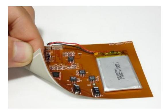
The completed monitor including power supply is compact and thin enough to wear under clothing.
