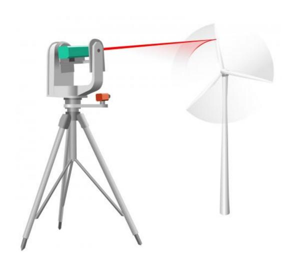
The laser tracks the motion of the rotor blades and remains exactly at the same position on the surface. Operators of wind turbines can measure the oscillatory pattern over the entire structure of the facility from several hundred meters away at every desired spot. Credit: Fraunhofer IOSB
