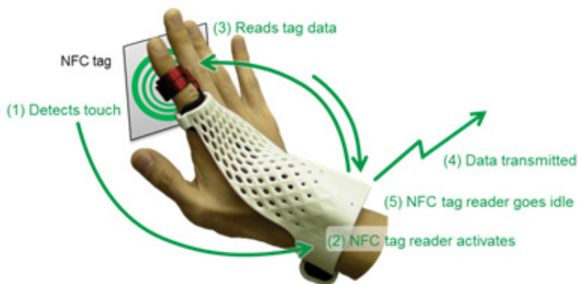
Figure 3: Steps involved in power-control operation
