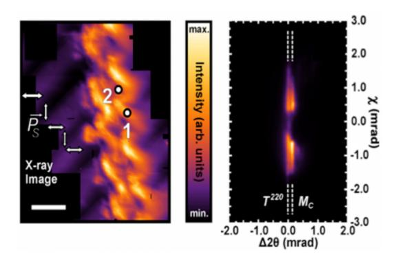
(left) Nanoscale scanning X-ray diffraction spatial map of the (220) Mc peak in BaTiO3 and (right) diffraction image of spot 2; scale bar 8 um. This projection image is of the entire structure, which exists a few microns into the material.
