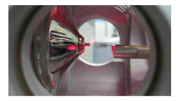
This equipment is used by Goddard's Astrobiology Analytical Lab to analyze very small samples. On the right is the nanoelectrospray emitter, which gives sample molecules an electric charge and transfers them to the inlet of the mass spectrometer (left), which identifies the molecules by their mass. Credit: Michael Callahan
