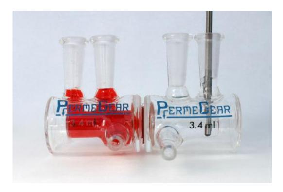
This experimental setup was used to test the properties of the graphene filters. A red dye in the water on left was used to demonstrate the filter's ability to block passage of the dye molecules.
