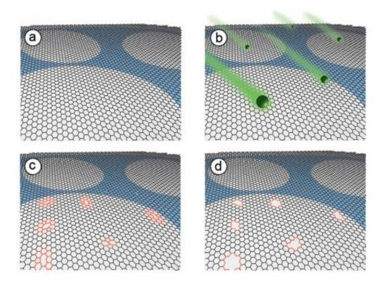
The MIT researchers used a four-step process to create filters from graphene (shown here): (a) a one-atom-thick sheet of graphene is placed on a supporting structure; (b) the graphene is bombarded with gallium ions; (c) wherever the gallium ions strike the graphene, they create defects in its structure; and (d) when etched with an oxidizing solution, each of those defects grows into a hole in the graphene sheet. The longer the material stays in the oxidizing bath, the larger the holes get.
