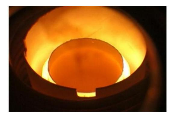
The new multicycle rapid thermal anneal technique reaches a peak temperature of 1350oC.
