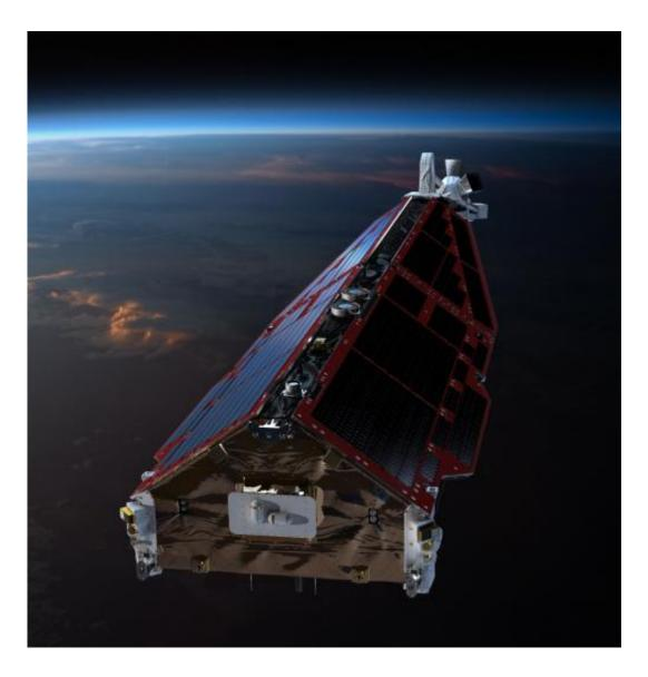
Swarm is ESA's first Earth observation constellation of satellites. The trio of identical satellites are designed to identify and measure precisely the different magnetic signals that make up Earth's magnetic field. The electrical field instrument, positioned at the front of each satellite, measures plasma density, drift and acceleration in high resolution to characterise the electric field around Earth. Credit: ESA/ATG medialab
