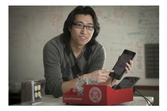
Li Jiang, a doctoral candidate in engineering, explains the solar thermal PCR test for a smartphone. The system can detect Kaposi's sarcoma - a deadly skin cancer related to HIV infection - in about a half-hour.
