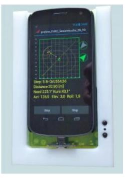
An extra piece of hardware coupled with the LawinenFon app transforms any smartphone into an avalanche transceiver. Pictured: the Galileo-LawinenFon prototype. Credit: Fraunhofer IML
