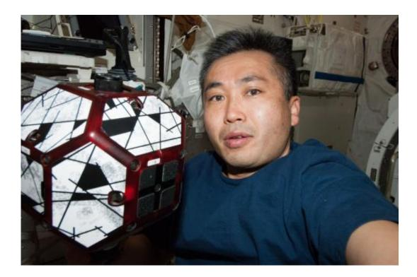
Japan Aerospace Exploration Agency astronaut Koichi Wakata, Expedition 38 flight engineer, conducting a session with a pair of bowling-ball-sized free-flying satellites known as Synchronized Position Hold, Engage, Reorient, Experimental Satellites (SPHERES) aboard the International Space Station. Credit: NASA
