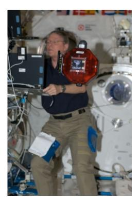
NASA astronaut Mike Fossum puts one of the Smart SPHERES through its paces during Expedition 29 aboard the International Space Station. The addition of the smartphone helped turn the SPHERES into mobile data acquisition assistants. Credit: NASA
