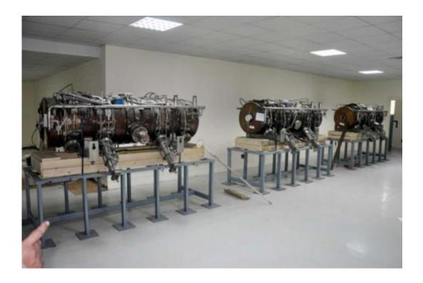
These radiofrequency cavities, built for the Large Electron-Positron Collider at CERN, will be re-used for training on the SESAME project. Credit: Sohail Janjua
