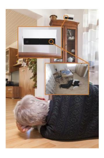
The sensor box registers the emergency situation in seconds and notifies the alarm unit in the home. Credit: Fraunhofer IPA
