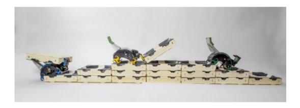
The TERMES robots can build themselves staircases to reach the next construction points, and they know how to add bricks that advance construction
