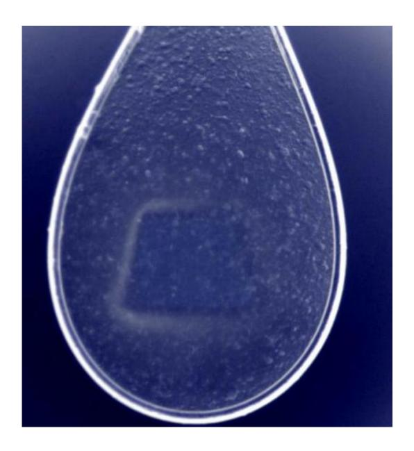
A nylon loop containing a thin film loaded with microcrystals. The X-ray beam scans the loop.
