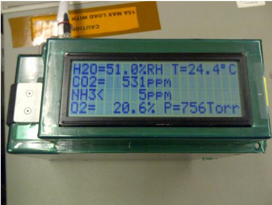
This is the Multi-Gas Monitor display showing four gas concentrations along with temperature and pressure. Credit: NASA
