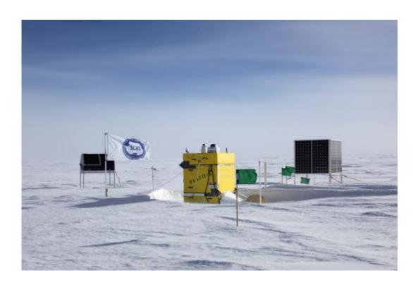
A UNSW-led team has used a telescope in Antarctica to identify a giant gas cloud in our galaxy which appears to be in an early stage of formation. Image is of the PLATO-R observatory at Ridge A. The HEAT telescope is the black object on stilts at left, the instrument module is the yellow box and the solar panel array is on the right. Credit: Geoff Sims
