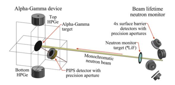
Laboratory set-up for testing the accuracy of the neutron monitor used in the "inbeam" method of measuring neutron lifetime.
