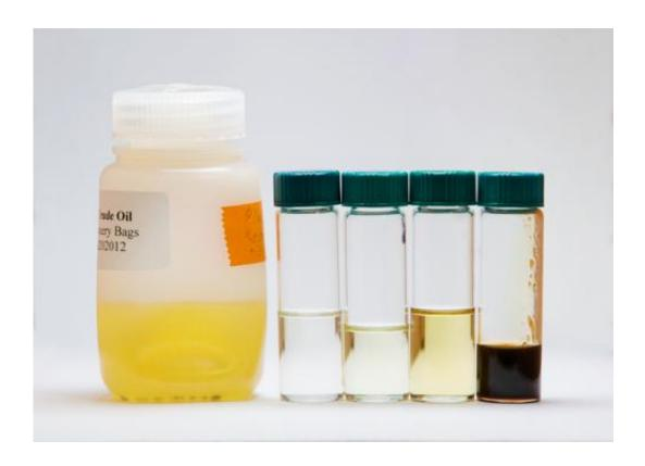
The team produced equivalents of (from left to right, in vials) gasoline, diesel #1, diesel #2, and vacuum gas oil. Credit: L. Brian Stauffer
