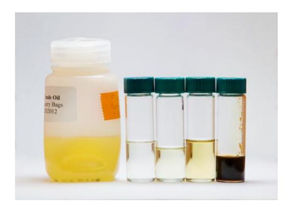
The team produced equivalents of (from left to right, in vials) gasoline, diesel #1, diesel #2, and vacuum gas oil. Credit: L. Brian Stauffer
