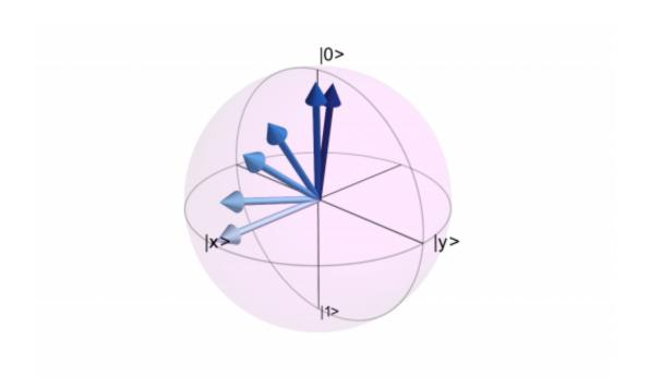
The state of the nuclear spin, visualised by the arrow, after measurements with varying strengths (light blue is very weak, dark blue is very strong). For increasing measurement strength, the state rotates towards the classical up state (arrow pointing up). This data is post-selected on one specific measurement outcome of the electron spin. For the other outcome, the arrow rotates downwards. Credit: Fundamental Research on Matter (FOM)
