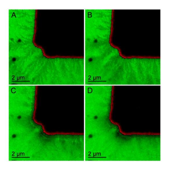
A new in situ transmission electron microscopy technique enabled ORNL researchers to image the snowflake-like growth of the solid electrolyte interphase from a working battery electrode. Credit: ORNL
