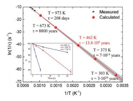
Arrhenius plot of the nanogratings decay rate at different temperatures. Black dots indicated measured values; red dots are calculated values. At a temperature of 462 K, the nanogratings would last for the current lifetime of the Universe. Credit: Zhang, et al. ©2014 American Physical Society
