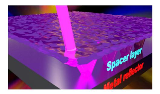
A rendering shows a beam of light interacting with an optical nanocavity. The nanocavity boosts light absorption in ultrathin semiconductors. Credit: Advanced Materials
