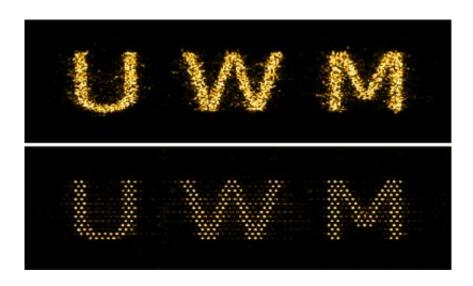
The images show the comparison between the simulated image transport through the researchers new optical fiber (top) with a commercially available endoscopy imaging fiber (bottom). Credit: Salman Karbasi
