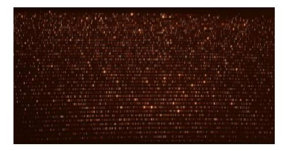
The dense spectral line structure of neutral thorium (Th I) as seen in a hollow cathode lamp observed with an echelle spectrograph. This is a double spectrum in which the visible spectrum is cut into horizontal strips to expand the wavelength range. Credit: Observatoire de Haute-Provence, France.
