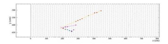
Data collected at the NOvA far detector in northern Minnesota shows one of the first interactions captured at that detector from a beam of man-made neutrinos. The neutrino beam is generated at Fermilab in Illinois and then sent through 500 miles of earth to the far detector. Credit: NOvA collaboration
