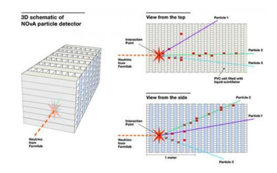
A graphic representation of one of the first neutrino interactions captured at the NOvA far detector in northern Minnesota. The dotted red line represents the neutrino beam, generated at Fermilab in Illinois and sent through 500 miles of earth to the far detector. The image on the left is a simplified 3-D view of the detector, the top right view shows the interaction from the top of the detector, and the bottom right view shows the interaction from the side of the detector. Credit: Fermilab
