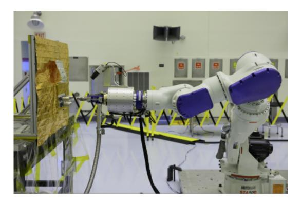
Located at Kennedy but commanded from Goddard, the RROxiTT industrial robot mimics how future space robots could transfer oxidizer to satellites that were not designed to be serviced. Credit: NASA/KSC
