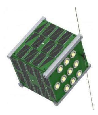
Solar arrays will charge the battery that aligns the satellite, powers its LED beacon, and sends radio messages about the health of its systems.
