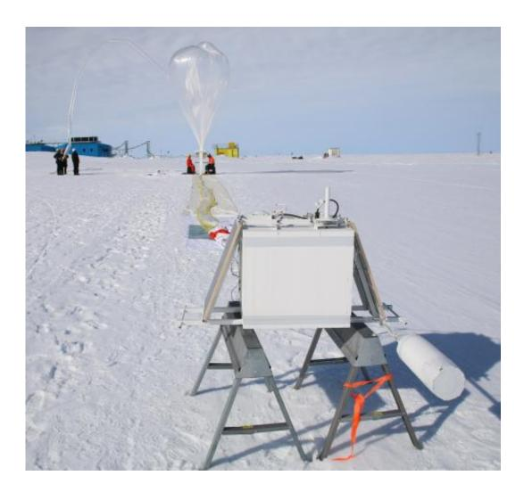
A BARREL balloon is inflated on Jan. 6, 2014 in front of Halley Research Station in Antarctica. The scientific payload is in the foreground and the parachute and balloon can be seen in the back. Credit: NASA/BARREL/Octavian Carp
