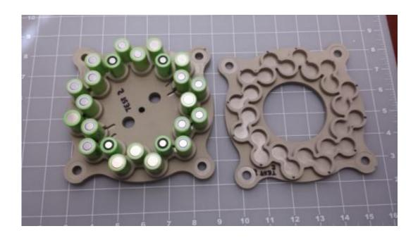
This battery case, created with a material called Polyetherketoneketone, is the first 3-D-printed component Goddard has flown. Developed under a university-industry partnership, the part was demonstrated during a sounding-rocket mission testing a thermal-control device developed with R&D funding. Credit: NASA
