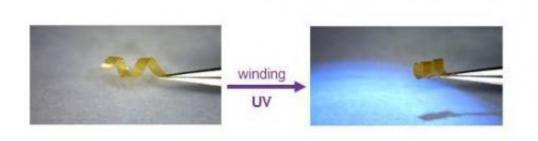
Researchers of the University of Twente's MESA+ research institute have developed spiral ribbons made of molecules, that are able to convert light into complex macroscopic motion. Therefore, they managed to amplify molecular motion and translate it to the macroscopic world. The research, which was inspired by movement in plants, is published in the major scientific journal *Nature Chemistry*.
