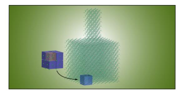
This shows an atomic-scale model of a nanophononic metamaterial. The vibrations caused by the pillar slow down the horizontal flow of heat through the thin film. Credit: Mahmoud Hussein
