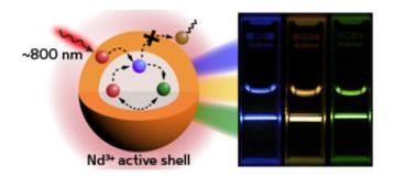
A core—shell nanoparticle can harvest light at biocompatible wavelengths (left) and produce luminescent light for bioimaging with tunable color emissions (right). Credit: American Chemical Society
